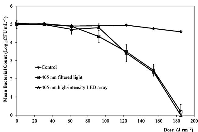
**Figure 4.** Comparative data for inactivation of *Listeria monocytogenes* through exposure to 405 nm filtered light (using xenon broadband light with a  $405(\pm 5) \text{ nm}$  bandpass filter), and a  $405(\pm 5) \text{ nm}$  high-intensity LED array, both with an irradiance of  $8.6 \text{ mW cm}^{-2}$ . No significant differences were observed between the inactivation kinetics for the light sources.
