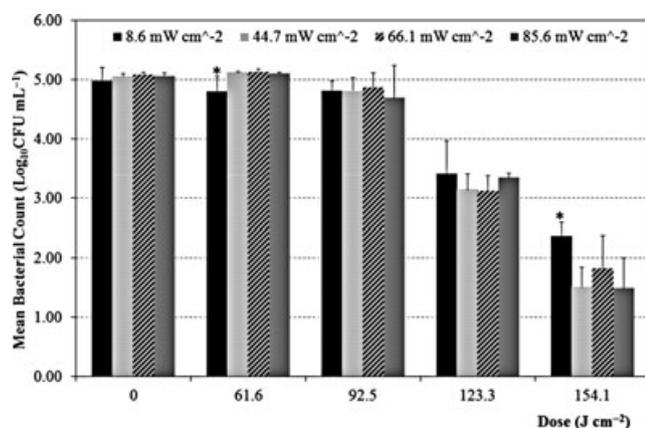
**Figure 5.** Dose-dependence experiments investigating the inactivation rates of *Listeria monocytogenes* following exposure to a 405 nm high-intensity LED array with differing irradiance levels. \* indicates where a light-exposed bacterial count was significantly different from the counts observed using the other irradiances at that particular applied dose ( $P \leq 0.05$  calculated at the 95% confidence interval).
