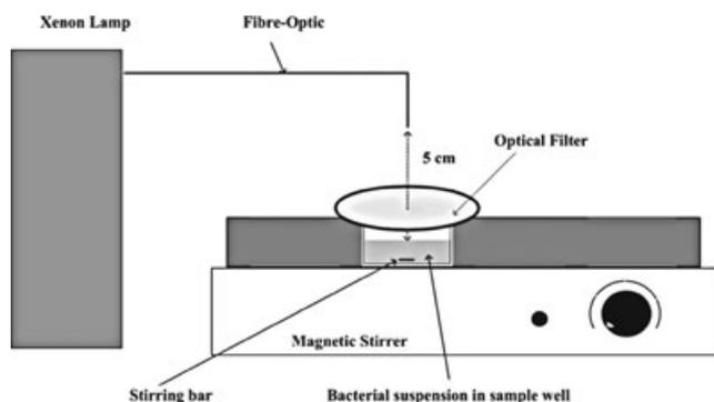
**Figure 1.** Experimental arrangement for investigation of the wavelength sensitivity of *Listeria monocytogenes*.
