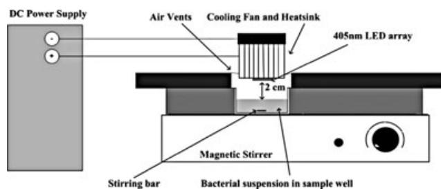
**Figure 2.** Experimental arrangement for inactivation of *Listeria monocytogenes* using high-intensity 405 nm light from an LED array.
